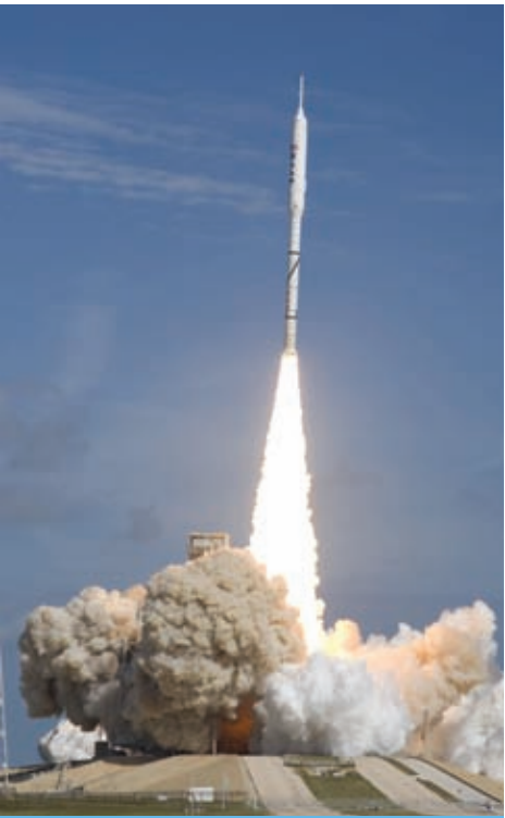
The Ares I-X produced 2.96 million pounds of thrust at liftoff. Photo courtesy of NASA
